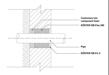
When sealing cable penetrations, jiggle the cables to reveal voids and re-press KÖSTER KB-Flex 200 into any eventual voids created. Ensure that the cable is tension free after finishing the sealing. Finally the sealing compound is recessed 1 - 5 cm (depending on cable thickness and weight) from the wall surface and smoothed with a metal spatula. As an additional safeguard and to hold the pipe / cable centered, the exposed material is covered with KÖSTER KB-Fix 5.
